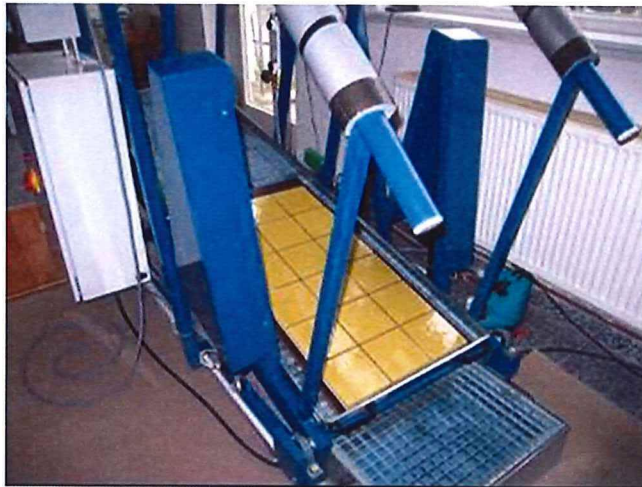
Fig. 2: Calibration board on Ramp test device
